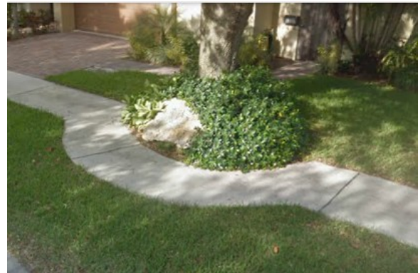
Routing the Sidewalk around canopy trees 200 Block of NE 13th Avenue
