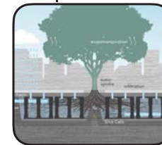
Resiliency - Silva Cells for Stormwater Management
