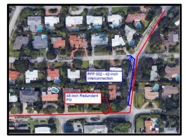
**Change Order No. 2.3 – RFP Item 5:** The MPC Team proposes the stub-out and valve will be placed 180 LF NE 14<sup>th</sup> Street. The connection orientation will be facing west.
