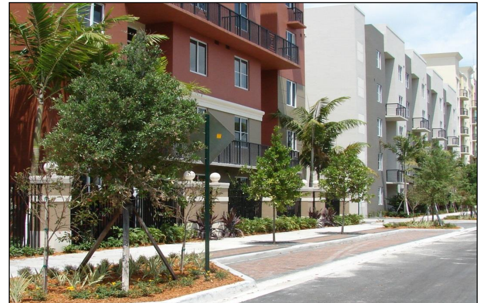
Figure 3.2, Example of street design with large shade trees in bulb outs, and small shade trees / ornamental trees in sidewalk
