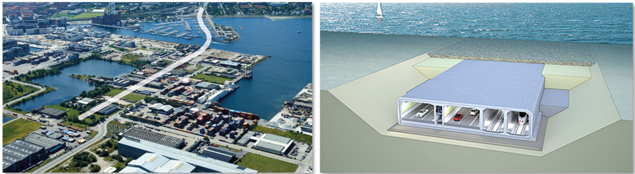
Exhibit 11 – Tunnel Unit Placed After Excavation
